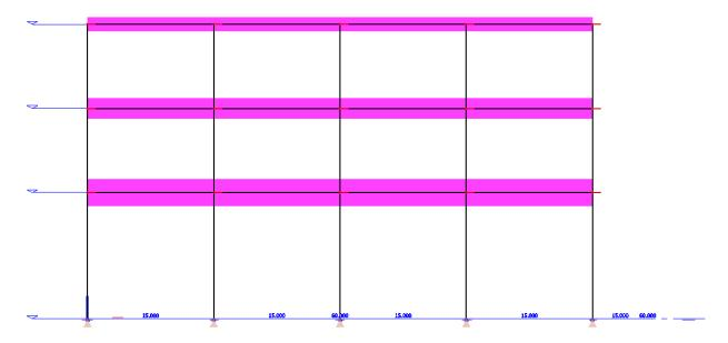
Once the masses are added to the model, a **K** Combination of mass groups should be created in order to combined all of the necessary masses that will be used for the Equivalent Lateral Force Procedure analysis.
